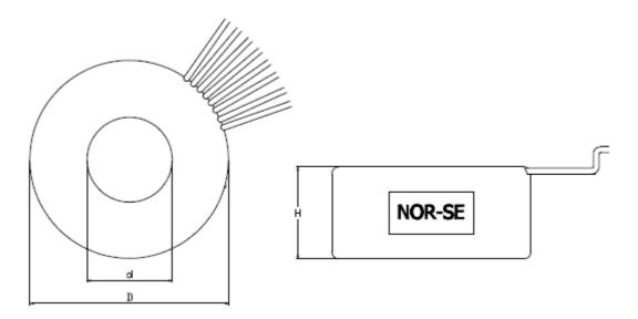
**Technical data:** 4-8 ohm and output 70-100.V **Frequency response:** 40-22000 Hz (+/- 3 dB) **Reference regulations:** EN 60065 (CEI 92-1)
