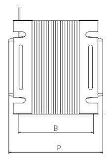
**Technical data:** 4-8 ohm and Output 70-100.V **Frequency response:** 80-18000 Hz (+/- 3 dB) **Reference regulations:** EN 60065 (CEI 92-1)
